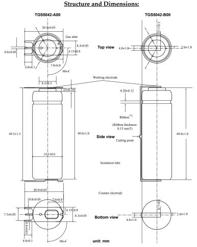
**NOTE\_1:** When the sensor is shipped, the working electrode and counter electrode are connected (i.e. short circuited) by a spring (-A00) or a metal ribbon (-B00) in order to avoid polarization of the electrodes. To measure the sensor outout, the spring should be removed (-A00) or the ribbon should be cut (-B00) and the sensor connected to a measuring circuit (*see example above*). The cutting point as indicated can be used to cut the ribbon easily.
