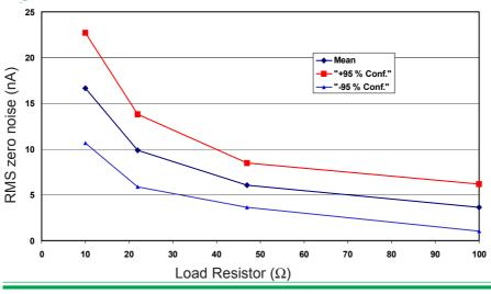
Figure 3 shows the effect of the load resistor on the RMS zero noise for the NO2-B1 sensor. The mean and ±95% confidence intervals are shown.
