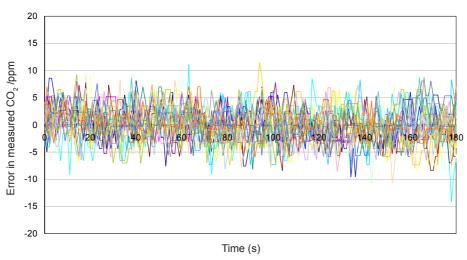
Excellent resolution and noise at 1000ppm CO<sub>2</sub> for the IRC-AT is achieved by better design, not by using more expensive components.
