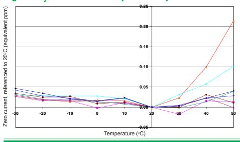
Figure 7 shows the variation in zero output caused by changes in temperature, expressed as ppm gas equivalent, referenced to the zero at 20°C.
