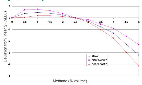
Figure 3 shows the nonlinearity from 0 to 5% methane (volume). Sensor non-linearity at 100% LEL is less than 4%.
