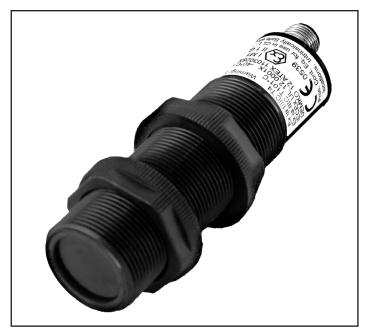
the maximum range of the unit. For example when using the RPS-409A-80-IS2, the output is a linear 0.125 V per inch. A target placed 10 inches from the sensor will result in an output of 1.25 V or a target placed at 80 inches from the sensor will result in an output of 10 V.
