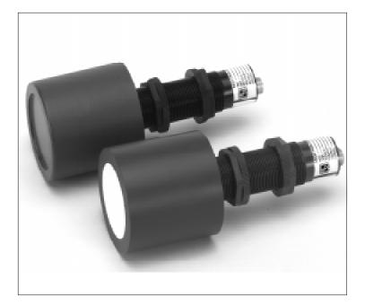
With the incorporation of a microcontroller into the design of the RPS-3000PVC and RPS-4000 many of the common problems facing long range sensing applications have been overcome. Software was then written optimize the performance to characteristics of the sensors. The artificial intelligence analyzes and conditions the return ultrasonic echo. This process filters out any false echoes and electrical noise. An additional task that the microcontroller does is temperature compensation.
