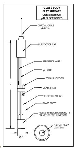
All electrodes are supplied with 30 inch cable and a BNC connector. Many other optional connectors are available for an additional charge.
