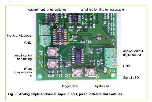
For basic operation close (ON) one of the switches 3, 4, 5 and both switches 6 and 7. The amplification can be selected as follows:
