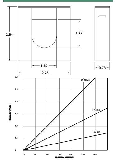
The **610-1000T** Split Core Current Transformer is designed for assembly to an existing electrical installation without the need for dismantling the primary bus or cables. It incorporates a snap fit between the fixed and removable sections.
