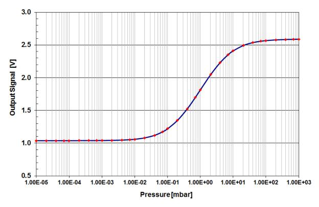
Output Signal versus Pressure in the range [10<sup>-5</sup>;10<sup>+3</sup>] mbar - Typical curve -
