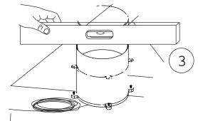
If the collector is not mounted absolutely level your readings will be incorrect.
