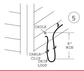
Run the wire into the house using insulated cable clips. Form a drip loop where the wire enters the house and caulk the feed thru hole when done
