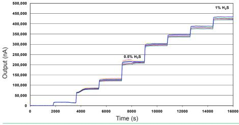
This sensor is built to withstand periodic high concentrations of H<sub>2</sub>S and recover without changing performance.
