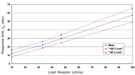
As with all Alphasense toxic gas sensors, increasing the load resistor slows the response time, but also reduces noise for better resolution.
