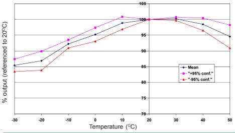
Figure 2 shows the variation in sensitivity caused by changes in temperature.
