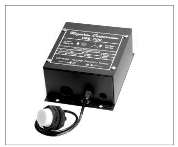
The RPS-300-T is a high frequency, sealed transducer unit best suited for environments where chemicals or weld splatter is a problem. The transducer head is constructed of a seamless Teflon body and sensing face. The remote transducer allows for mounting of the sensor head in cramped spaces while the controller is out of the way. The rang-
