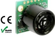
The LV-ProxSonar-EZ allows users to integrate several sensors into one system and experience little to no effect from the sensor interference than can occur with other ultrasonic sensor solutions. The LV-ProxSonar-EZ features an easy to use logic level (high/low) output, and RS232 format serial output. \*Factory calibration and testing is standard.
