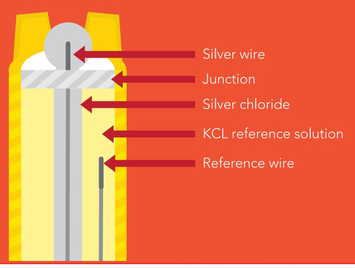
A pH electrode is a passive device that detects a current generated from hydrogen ion activity. This current (which can be positive or negative) is very weak and cannot be detected with a multimeter, or an analog to digital converter. This weak electrical signal can easily be disrupted and care should be taken to only use proper connectors and cables.
