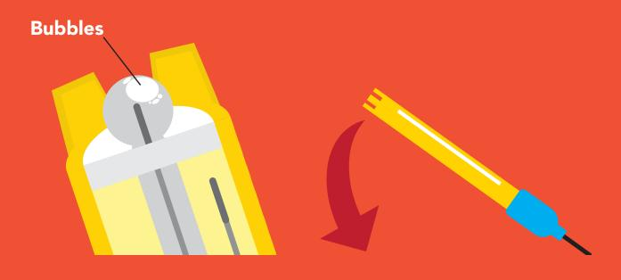
Vigorously stir the probe in the sample, calibration solution, or rinse solution.
