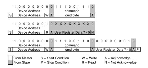
Figure 17: I<sup>2</sup>C read and write user register commands
