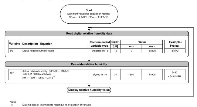
Figure 8: Flow chart for humidity reading.
