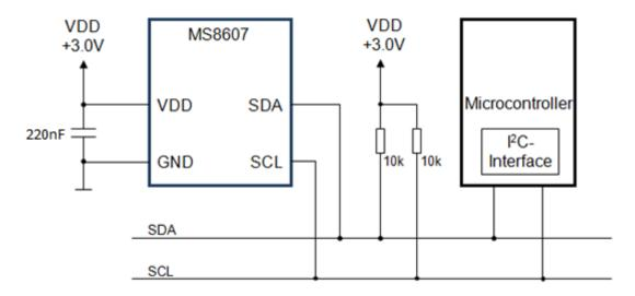
Figure 9: Typical application circuit
