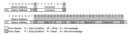
Figure 19: I<sup>2</sup>C Measure RH No Hold Master communication sequence
