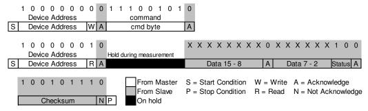
Figure 18: I<sup>2</sup>C Measure RH Hold Master communication sequence
