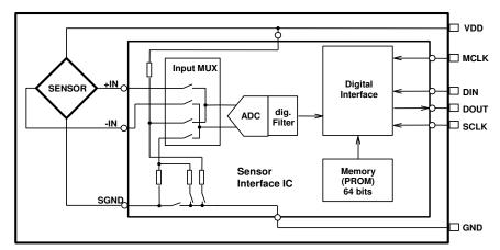
Fig. 1: Block diagram MS5536-60C
