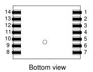
Fig. 2: Pin configuration of MS5536-60CPJU
