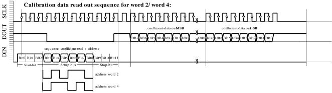
Fig. 6d: W2, W4 READING sequence
