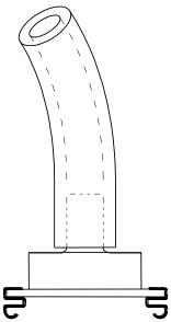
Fig. 10: connection to pressure port
