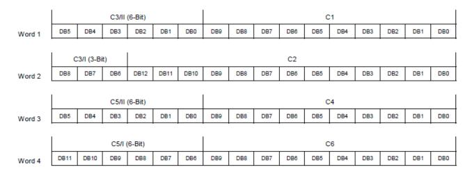
Fig. 4: Arrangement (Bit-pattern) of calibration data in Word1 to Word4
