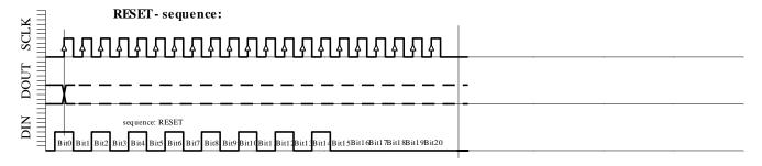
Fig. 6e: RESET sequence (21 bit)
