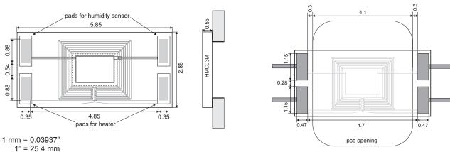
For shortest response time, in case of mounting onto a printed circuit board (PCB), HMC03M shall be positioned over an opening to allow enough air circulation around the sensor.
