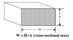
In a circular duct this cross section area equals the radius squared times  $\pi$  (3.14).
