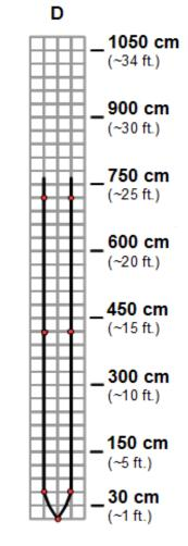
Beam Characteristics are Approximate Beam Patterns drawn to a 1:95 scale for easy comparison to our other products.
