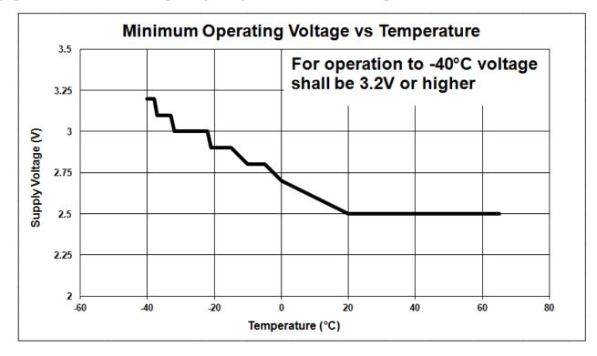
The graph below shows minimum operating voltage of the sensor verses temperature.
