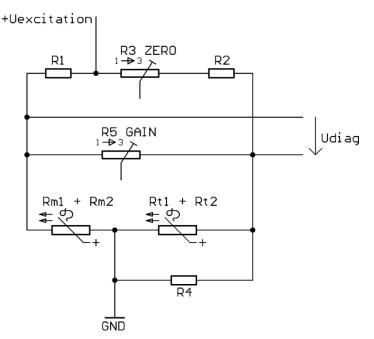
Fig.4: Application circuit for Wheatstone bridge operation
