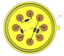
Fig.1: Pin assignment (top view)
