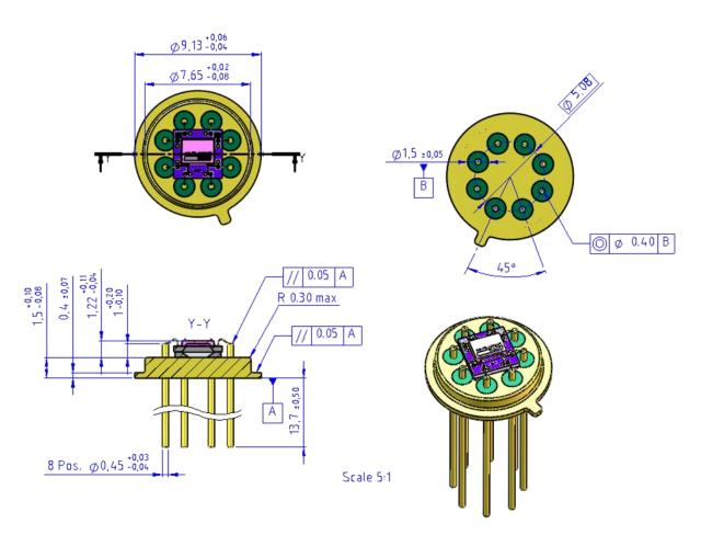
Fig.5: Mechanical dimensions (mm)
