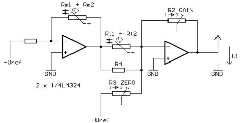
Fig.3: Application circuit for constant membrane current operation
