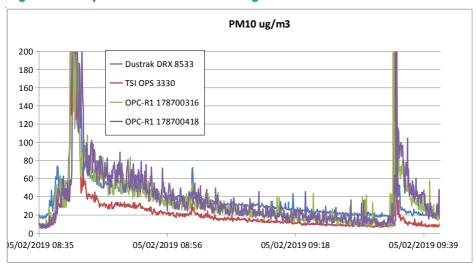
Figure 4 shows a comparison of PM10 monitoring by an OPC-R series sensor and TSI OPS 3330 and DustTrak instruments.
