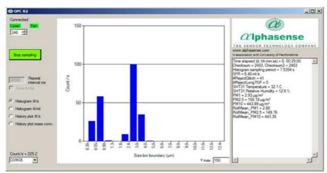
Figure 2 shows the OPC-R2 particle size distribution for the test aerosol.
