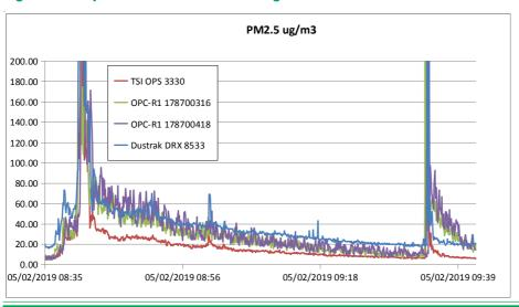
Figure 3 shows a comparison of PM2.5 monitoring by an OPC-R series sensor and TSI OPS 3330 and DustTrak instruments. All are set at 5s averaging and are sampling the ambient air of a work shop, the raw 3330 data has been used to calculate a PM figure.
