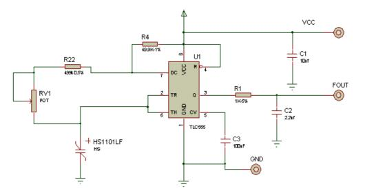
Note: R22=499k $\Omega$  / R4=49.9k $\Omega$  / R1=1 k $\Omega$  / RV1=50 k $\Omega$  potentiometer / C1=10nF / C2=2.2nF / C3=100nF
