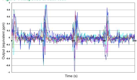
Simply breathing on a sensor causes both temperature and humidity transients.
