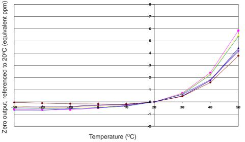
Figure 3 shows the variation in zero output caused by changes in temperature, expressed as ppm gas equivalent, referenced to zero at 20°C.
