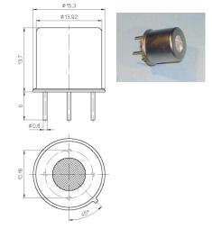
Screw mountable housings with sintered metal cap
