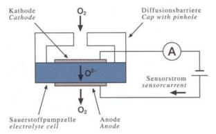
Schematic drawing of a sensor element
