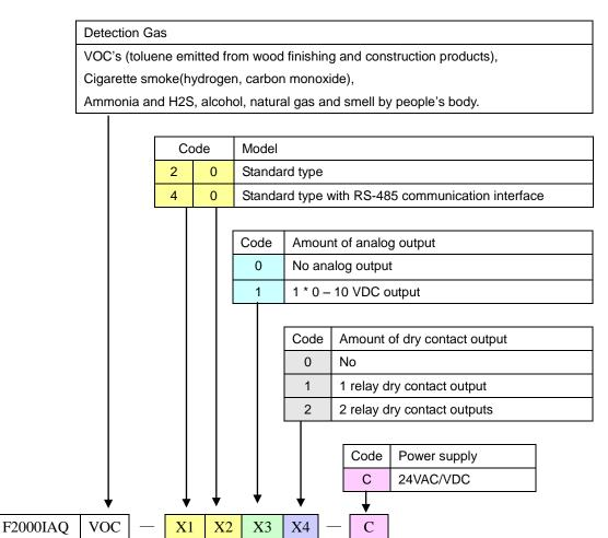
Example: F2000IAQ-VOC-2011 indicates the monitor can supply one analog output and one relay dry contact output.
