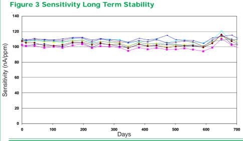
When sensors are tested monthly, their very good stability shows that they can be used in fixed sites, where maintenance and recalibration costs are important.
