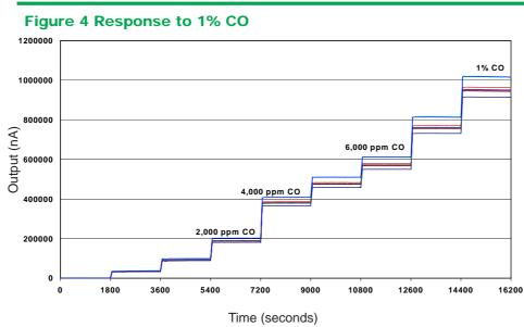
Figure 4 shows the response to step changes in CO concentrations from zero to 1% by volume.
