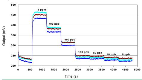
Figure 4 shows response from 0 to 1ppm CO.
