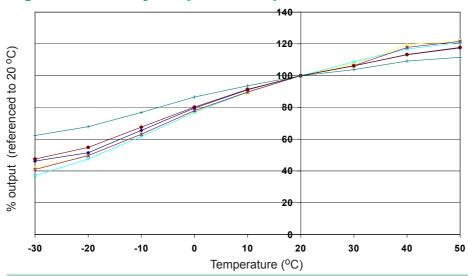
Figure 2 shows the temperature dependence of sensitivity at 2ppm CO.
