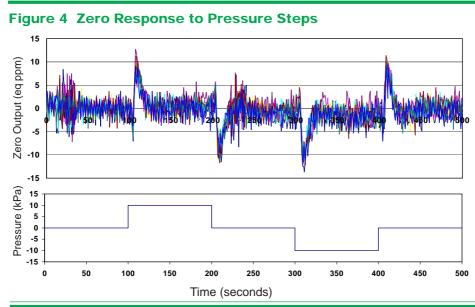
From ambient pressure, sensors were subjected to both positive and negative 10kPa pressure steps. The small transient rapidly decays as the sensor returns to its zero baseline.
