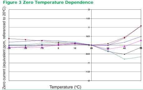
Figure 3 shows the variation in zero output caused by changes in temperature, expressed as ppm gas equivalent, referenced to zero at 20°C.
