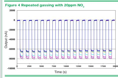
This hyteresis graph shows stable response when gassed repeatedly with 20ppm NO<sub>2</sub>
