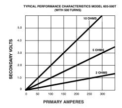
The **603 & 603D** Split Core Current Transformers are designed for assembly to an existing electrical installation without the need for dismantling the primary bus or cables.
