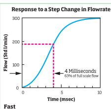
Fast 4 millisecond response ensures accuracy in fluctuating flows. This fast response is ideal for closed-loop control systems and integrated volume measurements. Pressure and temperature measurements are also extremely fast.
