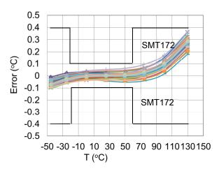
Accuracy vs. temperature (V<sub>CC</sub>=5V, TO18)
