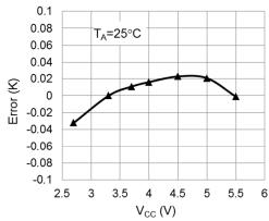
Normalized Error vs. Supply Voltage
