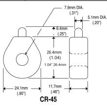
The CR45 Series, Wire Mounted Electrical Current Indicators provide an effective method of monitoring electrical current. The indicator is attached directly to a current-carrying wire. When the current exceeds the turn-on point, the LED will illuminate to indicate the presence of current.
