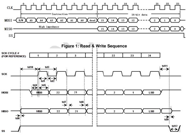
Figure 2: SPI Timing
