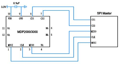
Note: the capacitors should be placed as close as possible to the VDD pin
