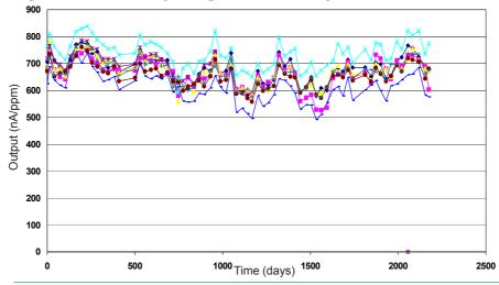
Figure 4 shows the excellent long term stability of the H2S-A1, which results from the combination of a patented design, superior electrochemistry and good process control.
