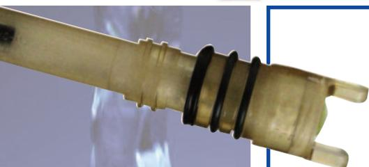
**2005145** – This **General Purpose Electrode** has a two tine Radel body, double junction reference and slightly radiused pH bulb. While suitable for higher temperatures it is optimized for fast and stable readings in ambient temperature applications. Neutralizations, waste effluent monitoring, rinse applications and potable water are just a few of the suggested applications.
