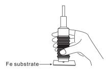
c. Do not lift the detect tip and press the "▲" and "▼" key to adjust the reading as same with the standard piece, after these calibration is complete, the instrument is ready to use. LCD displayed like the following picture:
