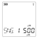
Press "(wit)" key, you can select your desired unit on um to umil, LCD displays as shown below:
