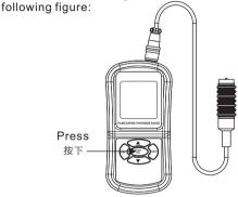
3. After the entire screen displays for 1 second, the default state is single test mode .if the LCD screen displays the symbol or or , please promptly replace the battery, as shown in following figure:
