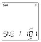
Contact detect head with the test surface vertically and press the detect head lightly, LCD displays a value, for example, 109 μm, and buzzer sounded at this time, LCD displays as shown below:
