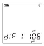
Place the sensor head to the target piece you want to measure, then press the detect head lightly to measure, the buzzer beeps, LCD will display the value of the difference between the last reading and the current reading, LCD displays as shown below:
