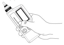
b. After the entire screen displays for 1 second, the default state is acceleration mode, if on the LCD displays the symbol or , please promptly replace the battery, as shown in following figure:
