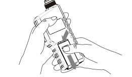
b. Insert a 9V battery into battery compartment, note the battery polarity, and then close the battery door, as shown in following figure:
