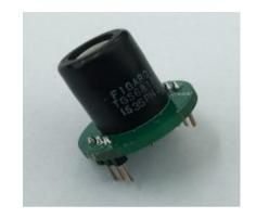
Furthermore, the unit can detect CH4, LPG, H2. It is less sensitivity to VOCs gas, it immunes poison by silicon compounds, it suits to work at rugged environment.
