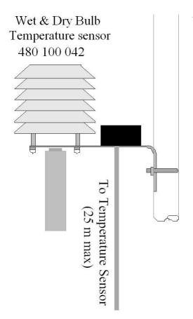
Wall or mast mount away from heater or air conditioner outlets.
