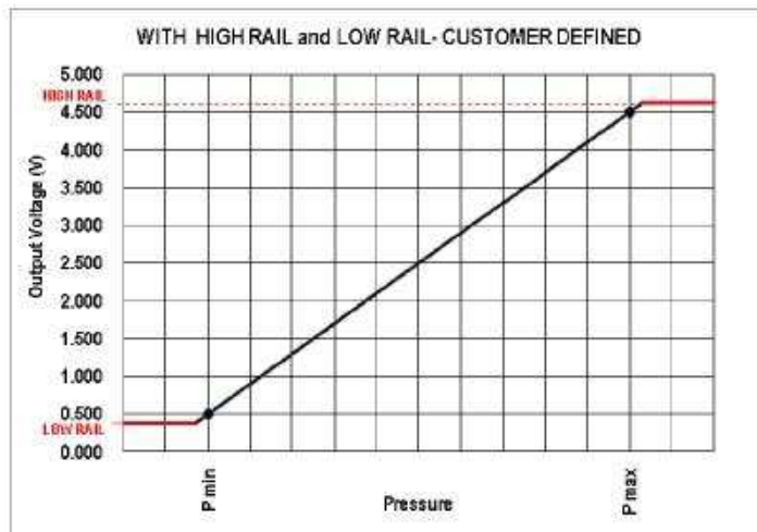
CHART B. OEM CUSTOM CALIBRATION. HIGH / LOW RAIL VALUES CAN BE ADJUSTED BY CIRCUIT
