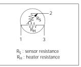
Fig 1d. Equivalent circuit
