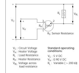
Fig 2. Standard circuit
