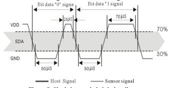
Figure 8: Single bus exploded timing diagram
