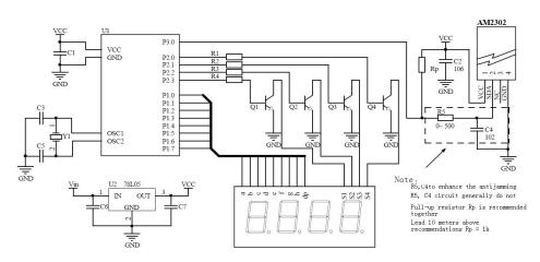
Figure 4: AM2306 single bus typical circuit
