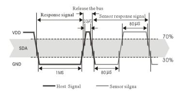
Figure 7: Single bus exploded timing diagram
