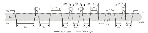
Figure 6: AM2306 single bus communication timing
