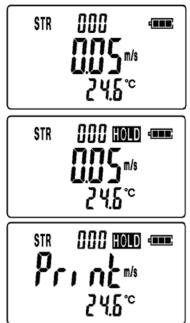
Hold the reading by pressing the  $\frac{\text{ENTER}}{\text{HOLD}}$  key.
