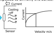
the air velocity and the resistance value (Platinum Coil) is known, the air velocity can be obtained by measuring the resistance value (or current).
