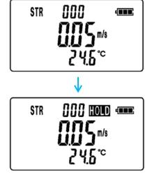
While measuring, press the  $\frac{\text{ENTER}}{\text{HOLD}}$  key to hold the current reading.
