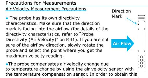
compensation effect, it is required that both sensors are evenly exposed to the airflow under the same temperature conditions.
