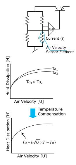
The Anemomaster anemometer is based on the above principle. Generally, a hot-wire anemometer employs a feedback circuit to control the sensor to maintain constant temperature. (Constant Temperature Type)
