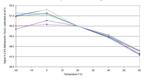
Effect of Temperature on Zero Signal
