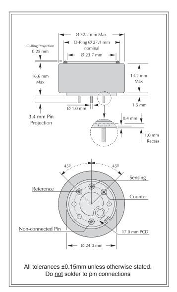
**IMPORTANT NOTE**: Connection should be made via PCB sockets only. Soldering to the pins will render your warranty void.
