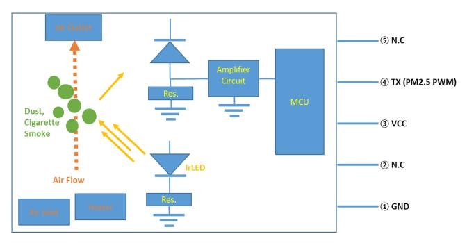
Figure 2. Example of Internal Schematic
